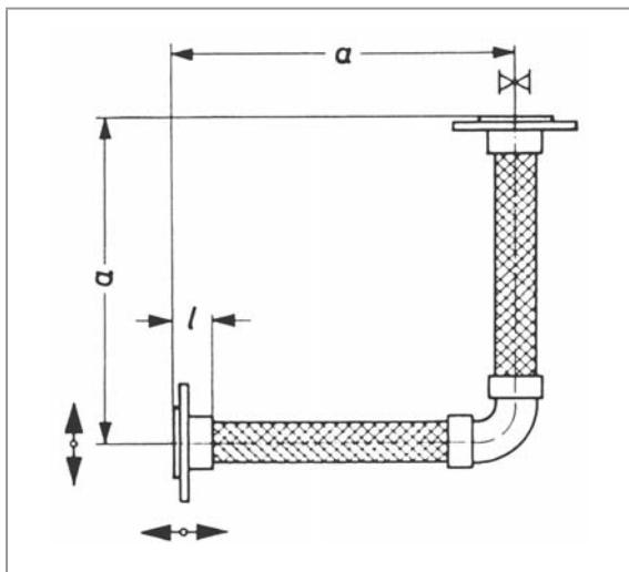
Permissible amplitude at permanent load:
